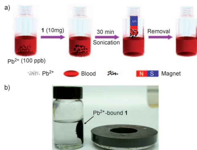
Figure 5. a) Illustration of the removal of Pb 2+ from human blood. b) Photograph of a magnet attracting Pb 2+ -bound 1 in water.
